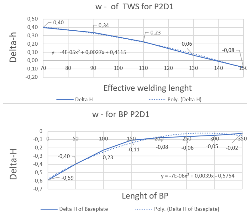
Figure 68: Delta-h of P2D1 described by an estimated second degree polynomial of TWS and BP.
