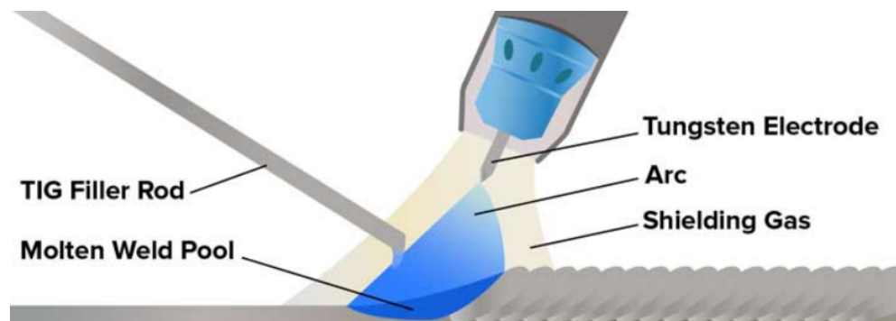
Figure 2: TIG welding process. Source: [8].
