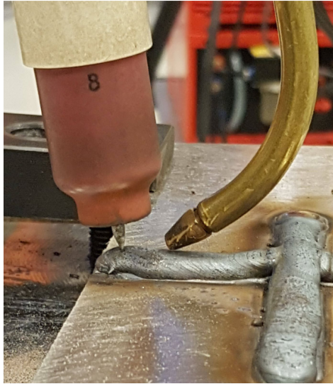
Figure 38: Tungsten electrode crash in sample P2D2. Source: Picture from the welding experiment
