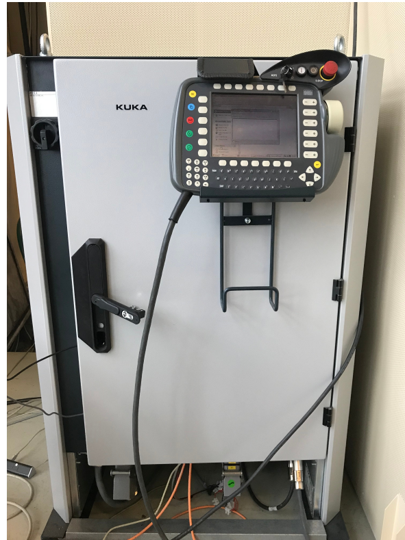
Figure 9: A picture of the KUKA KR C2 controller that is used to control the KUKA KR 30-3 robot.
