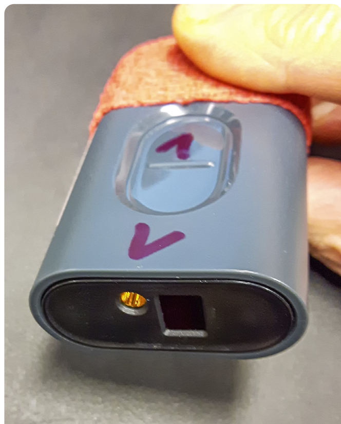
Figure 4 The mobile NIR spectrometer. The yellow field to the left is the light source. The incoming radiation is then partly absorbed in the probe and scattered. Only a fraction of the reflected light reaches the sensor to the right and the rest is absorbed or lost.
