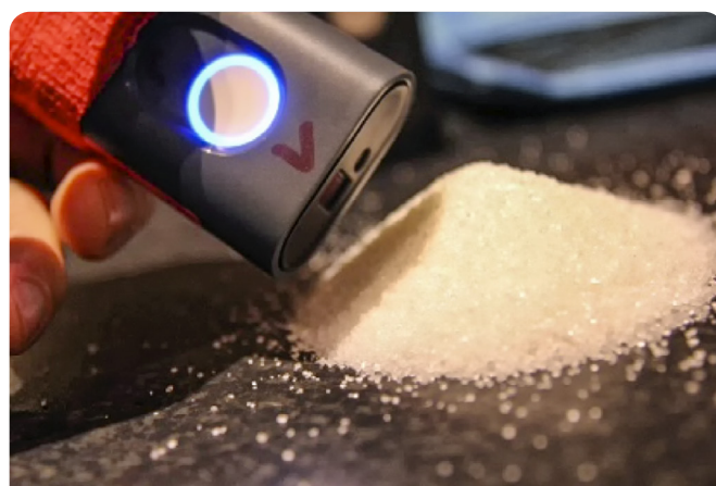
Figure 1 Using a mobile near-infrared spectrometer in the classroom
