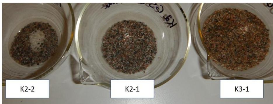
**Figure 5.2.** The lithology distribution of the diamict K3-1 shows a higher distribution of red granite in comparison the diamicts K2-1 and K2-2.
