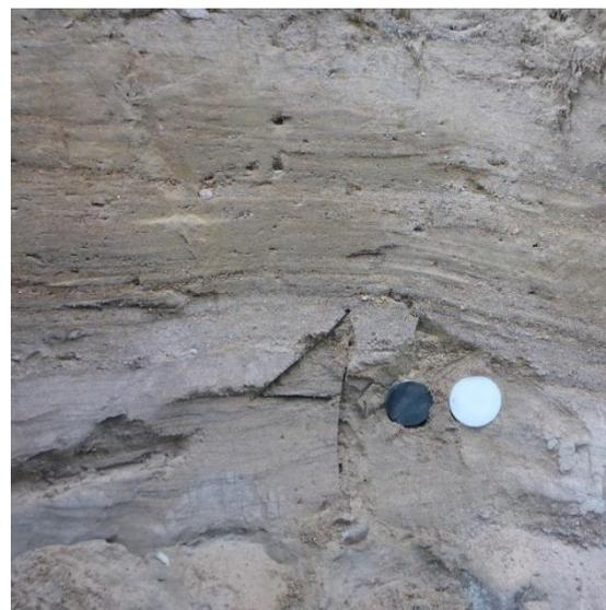
**Figure 3.4.** The OSL samples and the background samples from the western ridge were collected in opaque grey plastic tubes (black lid). The water content and density were measured from material collected in cylinder volumeters (white lid). Photo by Helena Alexanderson (2018).
