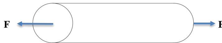
Figure 10 - Tie rod, subject to tension
