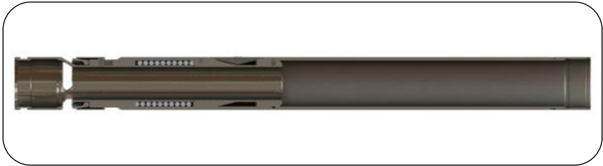
Figure 21 - FEMF - Version 3 - Section view of the actuator sleeve, seal and centralizing mechanisms
