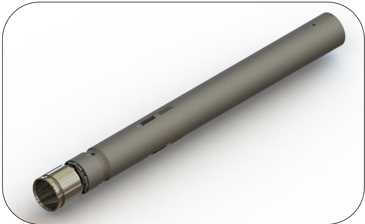
Figure 20 - Concept 1 - Force-Expanded Metal Flaps (FEMF) - Version 3
