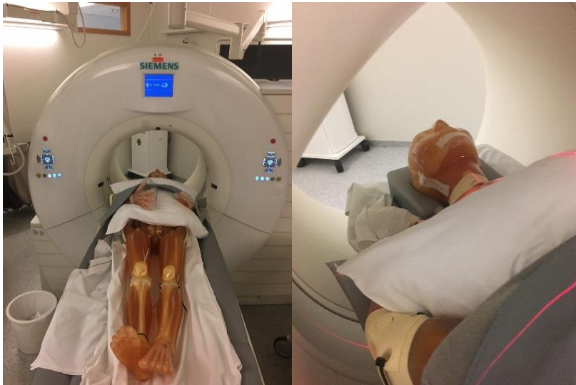
CT whole-body phantom PBU-60 Kyoto Kagaku in scan position in CT machine in room 12 and 7. Machine name Siemens Somatom definition flash. Scan date 09.05.18
