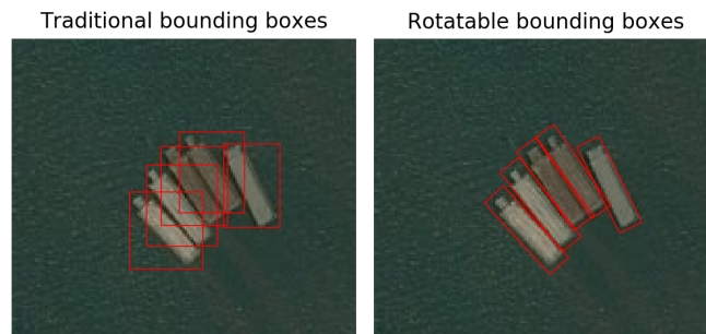
Figure 5.4: Image tile visualizing how the RBox is able to locate the ship more precisely, while excluding background from the bounding box, as compared to the traditional BBox. Image is from the Airbus ship detection data set (Kaggle, 2018).
