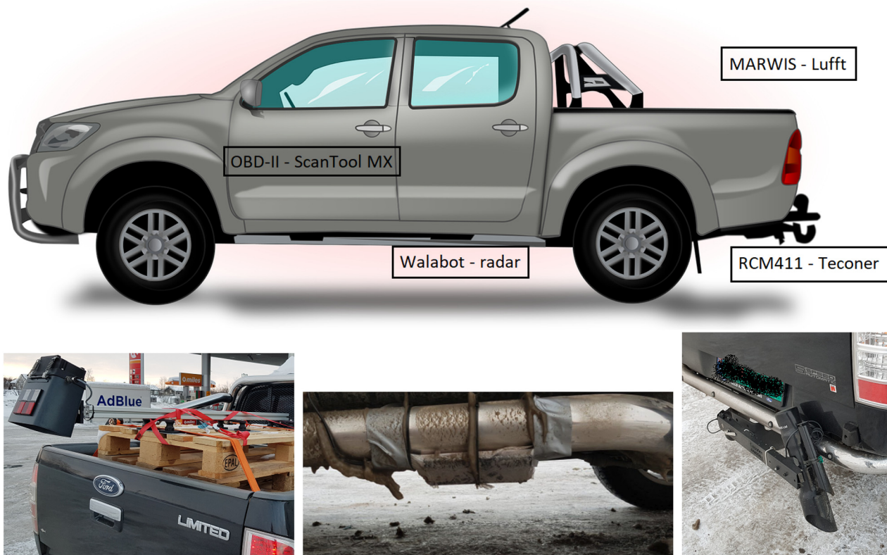
Fig. 2. Placement of the sensors on the car. Top image by OpenClipart-Vectors from Pixabay.
