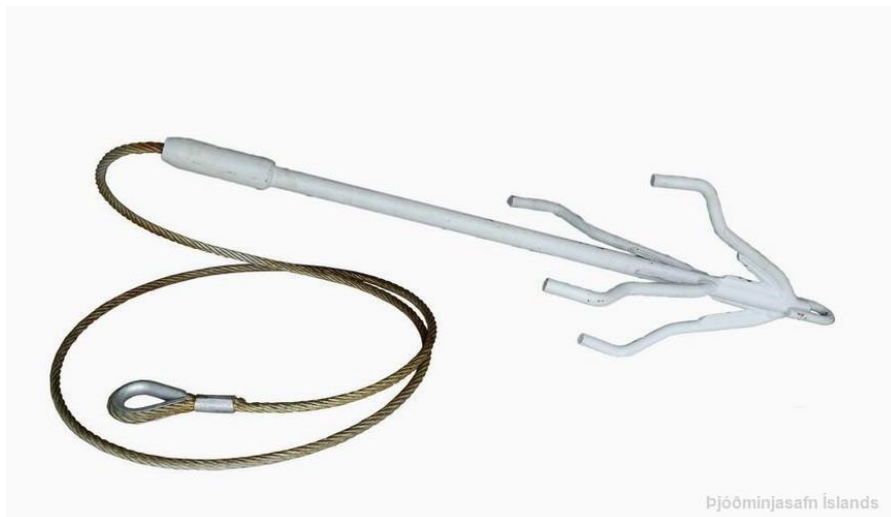
Picture 1 Net wire cutters used to cut nets of foreign vessels (Þjóðminjasafn Íslands, n.d.)
