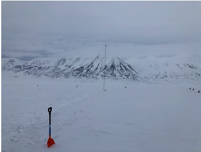
Figure 5.2: The transmit antenna at TX location. Diamond WD330 25 m folded dipole, setup as an inverted-V.
