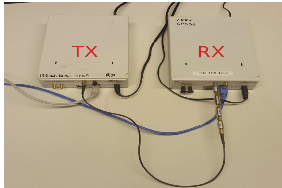
Figure 4.3: Setup of the transmitting USRP labeled TX and the receiving USRP labelled RX. The RX has 3 additional attenuators and a DC block connected to the input port.
