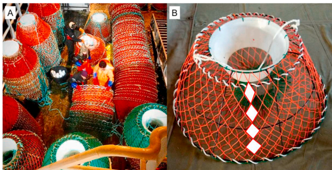
Fig. 1. A: Barents Sea snow crab vessel (MS North Eastern) on its way to the fishing grounds with the deck full of stacked conical pots (Photo: Opilio AS); B: differences in mesh opening angles along the height of the traditional conical pot.
