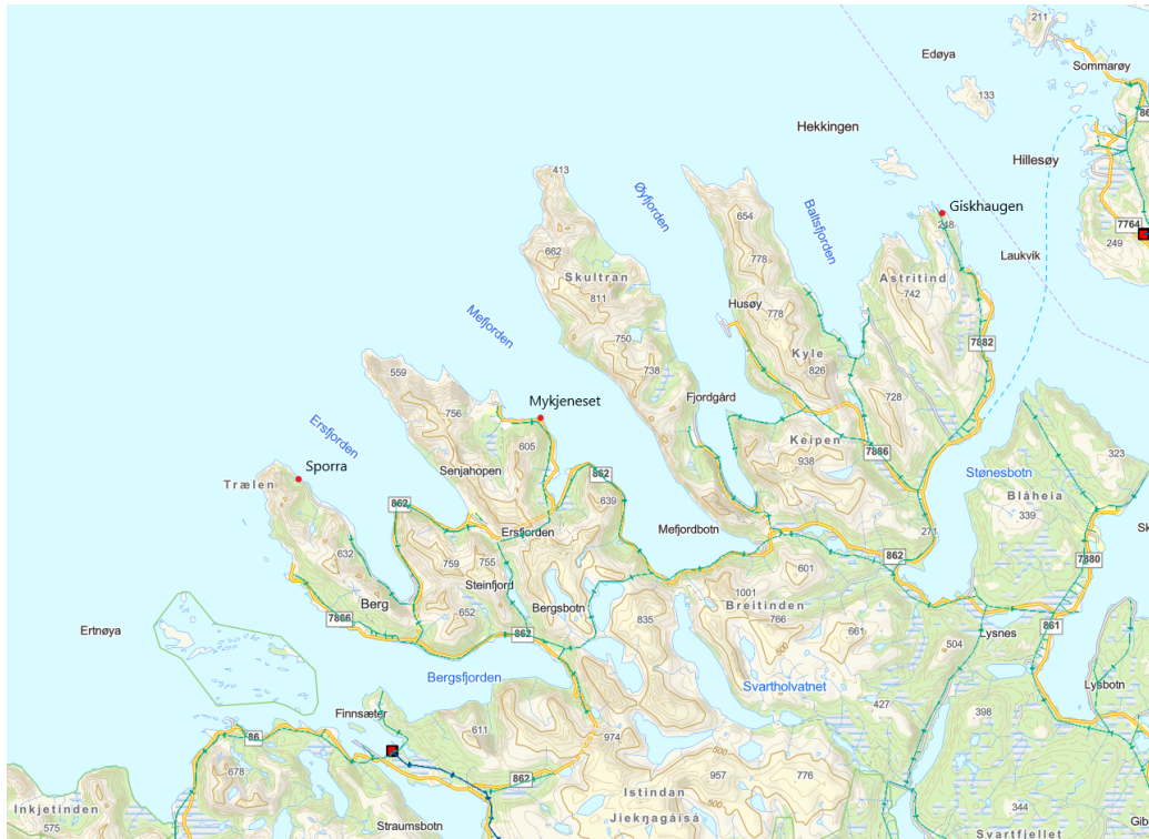
Figure 4.10: Topography map of northern Senja which show the existing 22kV , and 132kV power lines as green, and blue lines, respectively. The red boxes are transformer stations, and yellow solid lines are main roads.
