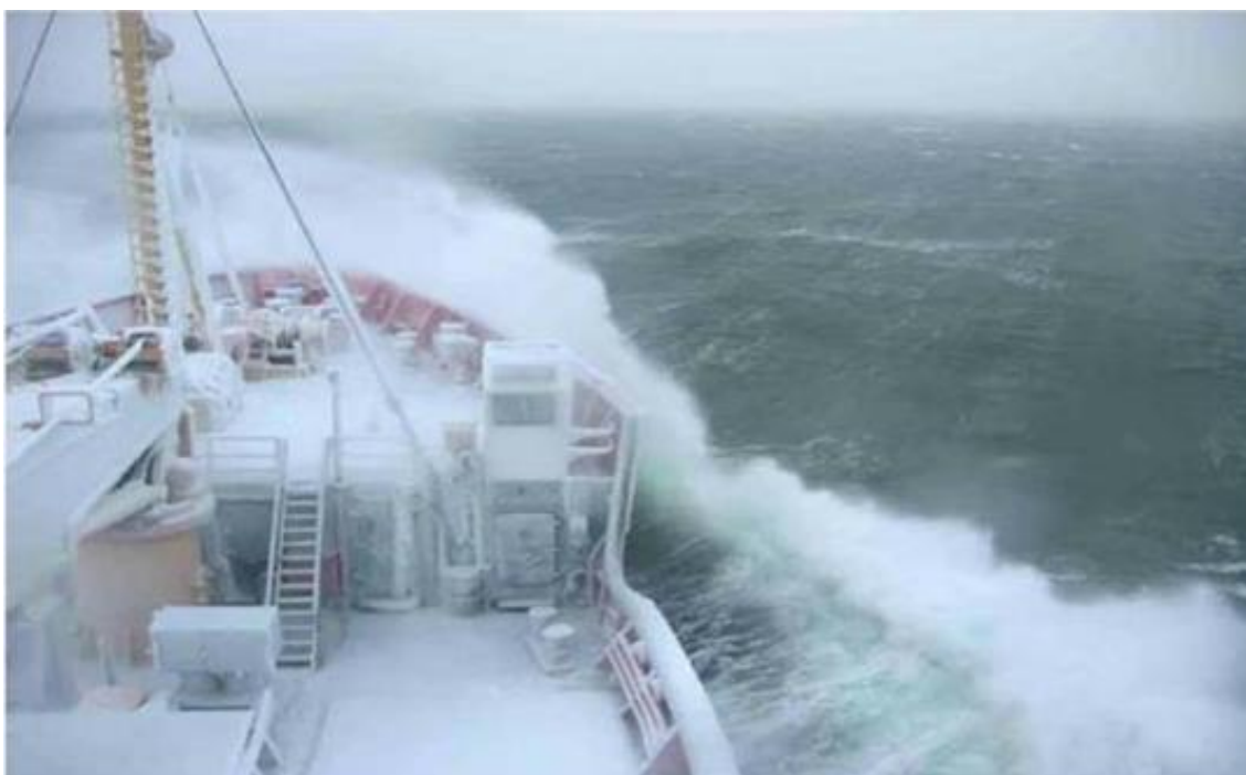
Figure 1. Icing due to the collision of ship and waves (Toomey, Lloyd, House, & Dickins, 2010)
