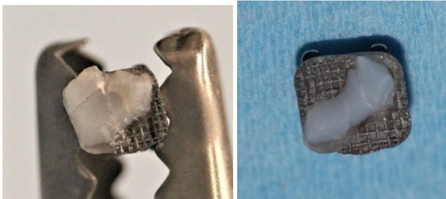
Fig.6 (A, B) Excluded stainless-steel sample A: Substantially thicker adhesive material compared to the other samples before sandblasting. B: The excluded sample after sandblasting and the test parameters were far from enough to remove adhesive material.
