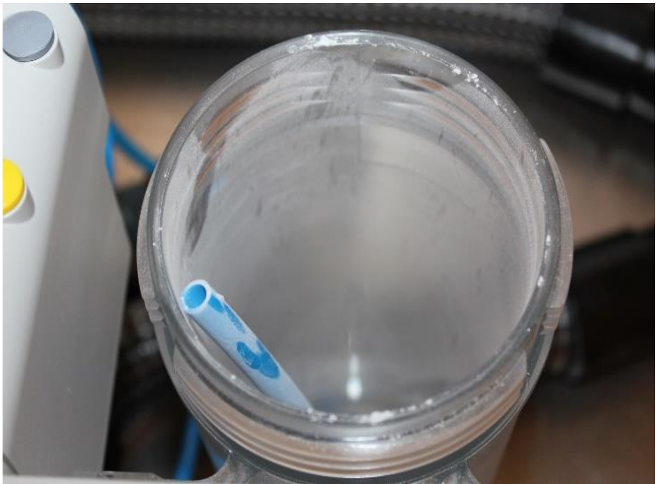
Fig. 9 Empty container for abrasive material (aluminium oxide) of sandblasting machine.
