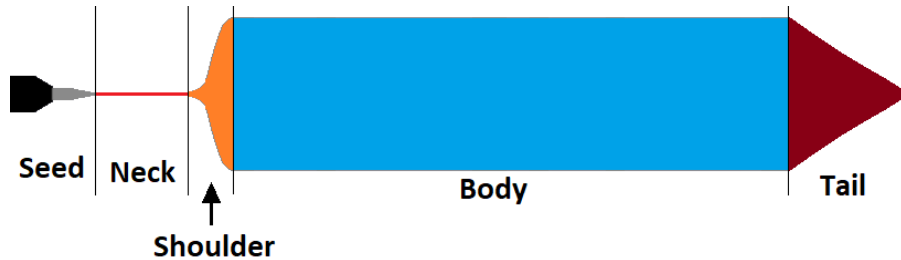
Figure 24: Labeled illustration of the sections of a finished boule
