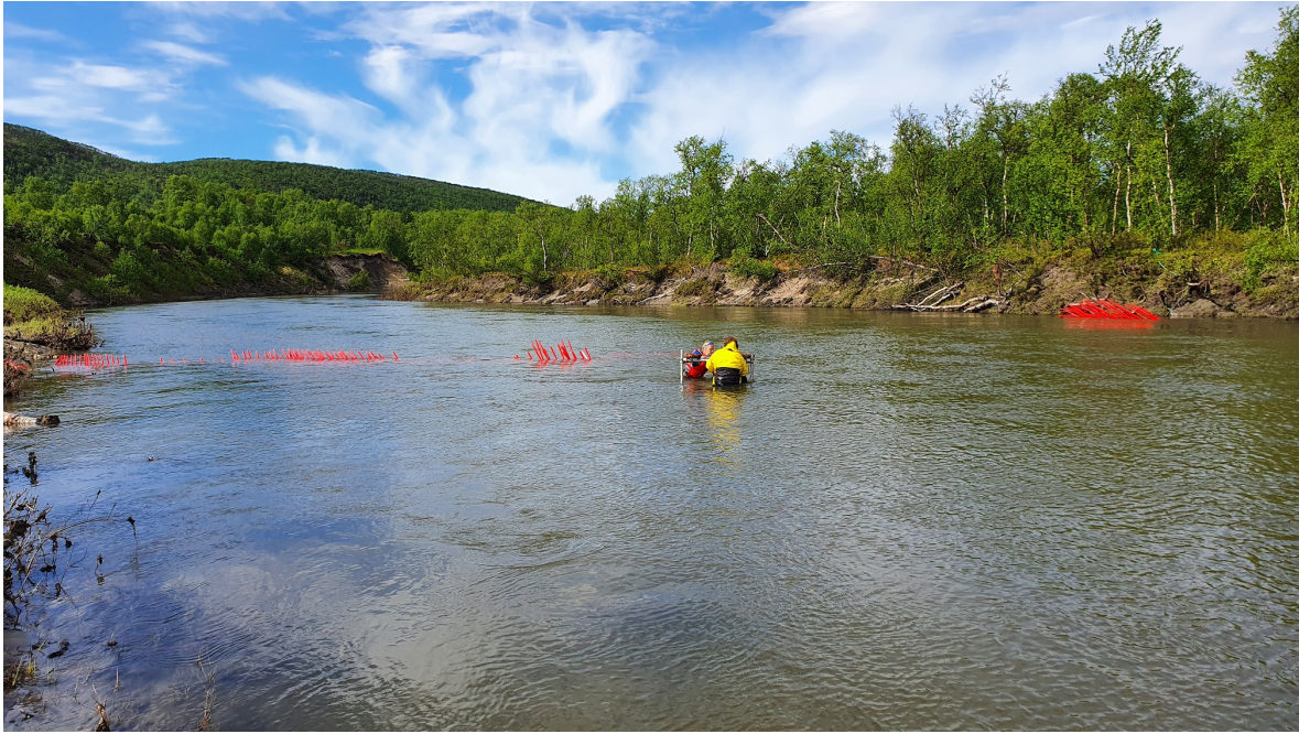
Figure 4. Placement of sonar in Måskejohka. Red guiding fences from both shores narrows the fish passage. Photo: N. S. Johansen.
