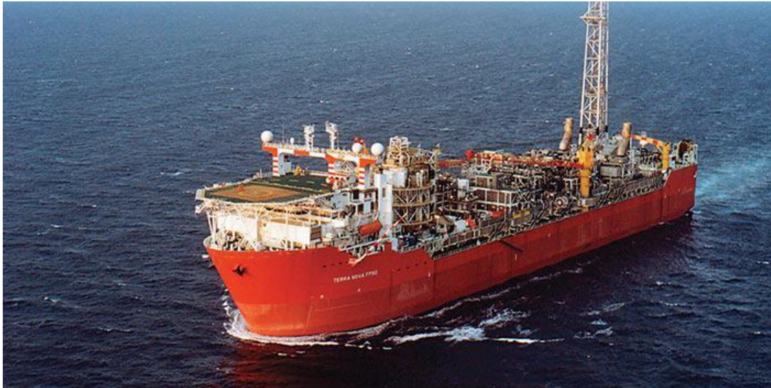
Figure 22. 'Terra Nova' is another FPSO, used in the Canadian Arctic region. 350 kilometres southeast of Newfoundland and Labrador, Canada, is one of the largest FPSO vessels ever built, at a length of 292.2 metres, a width of 45.5 metres and it stands more than 18 storeys high. The FPSO can store 960,000 barrels of oil and accommodate up to 120 personnel. Source: https://petro-canada.com/en-en/knowledge-centre/casestudy/terra-nova
