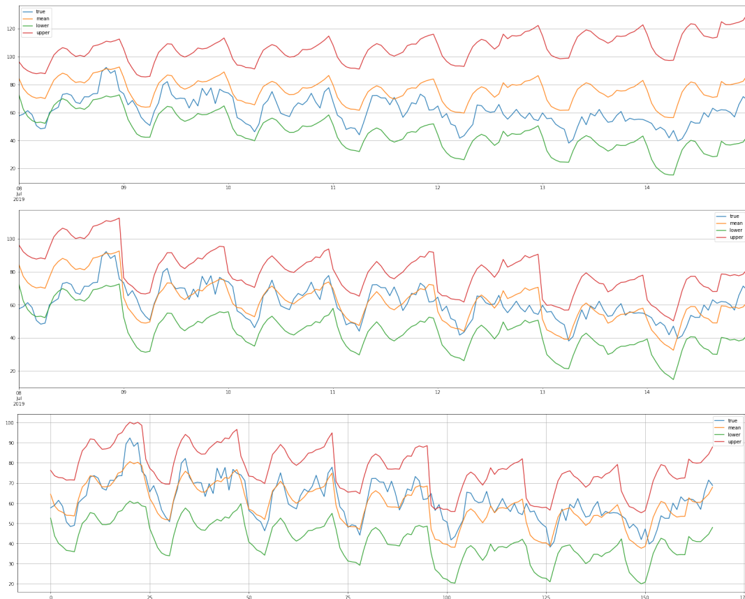
Figure 30: Illustrations of a SARIMA model producing wide and shifted prediction intervals. The plots show three models fitted using the Household time series from the Elvia dataset, with training data from 1 June 2018 to 31 May 2019. All models predict test observations from 8-14 July 2019. The model in the top plot is not presented with new data after being fitted, and predicts all test observations at once. The model in the middle plot predicts 24 hours ahead for each day in the test data, and is presented with the actual observations after the predictions are made. However, the observations from 1-31 June 2019 are not presented to the model and, thus, it performs poorly in the beginning. In the bottom plot, the model is presented with observations from 1 June to 31 June 2019 after being fitted, as well as the actual observations after the predictions are made. The prediction interval is no longer shifted as before, since the model is presented with all required data. The blue line corresponds to the actual observations, the yellow line is the predicted mean, and the red and blue lines represent the upper and lower prediction interval bounds, respectively.
