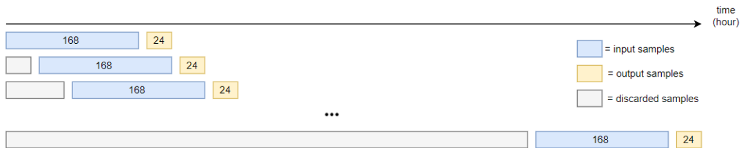
Figure 18: Predictive setup using sample pairs with input and output size of 168 and 24, respectively. Total sample length = 192 hours.
