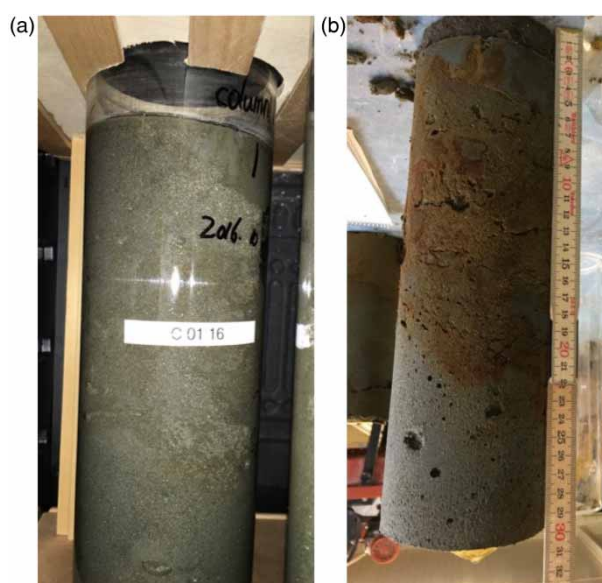
Figure 3 | (a) The column run at 5 °C a few weeks after the leaching experiment had started and (b) the same column at the end of the leaching experiment (taken out of the acrylic-plastic column). The column has a 2 cm layer of sludge material on top.
