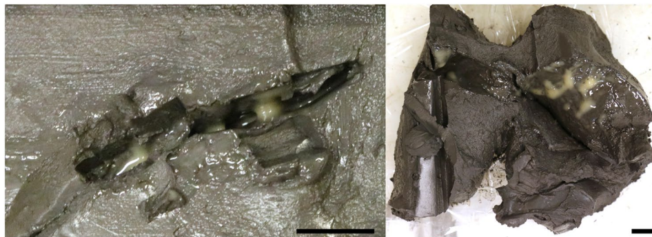
Figure 2. Sediment core GC1048 with biofilm pocket after retrieval, cutting the core into half and sampling. Scale bars = 1 cm.
