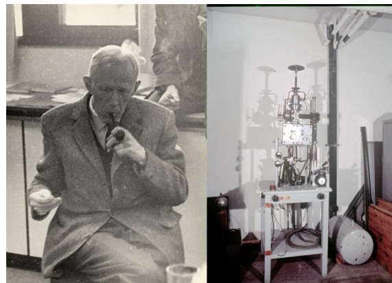
Figure 1. Left: Odd Hassel smoking a pipe at Blindern campus, Oslo. Right: Gas-phase electron diffraction apparatus constructed by Hassel and co-workers. Photographers: unknown . [6]
