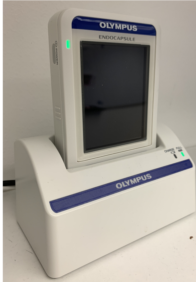
Figure 2.7: Olypmpus RE-10 endocapsule recorder used in our data collection for Kvasir-Capsule [180]
