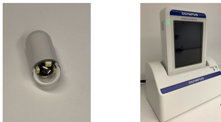
(a) Olympus EC-S10 endocapsule (b) Olympus RE-10 endocapsule recorder
