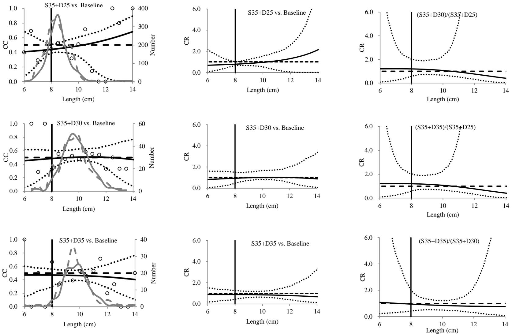
**Fig. 3.** Catch comparison rate (CC, first column), catch ratio (CR, second column) and catch ratio comparison (CR, third column) curves of the three CSDM cod ends for greasyback shrimp. The circle marks represent the experimental rates. The thin dotted curves
