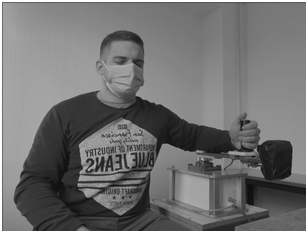
Figure 1. The motor-driven proprioceptor used for the measurements
