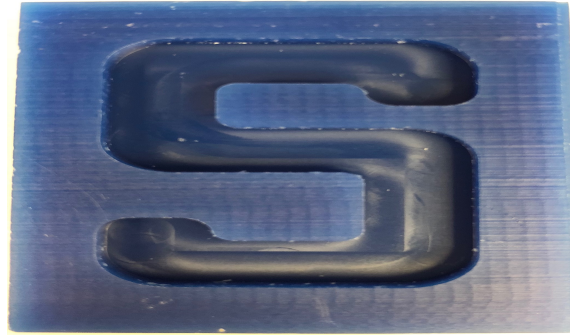
Figure 4.1: A wax block that has an S-shaped curve to it. The wax block is a part of the CNC Mill Tool Wear dataset. Sun (2021)
