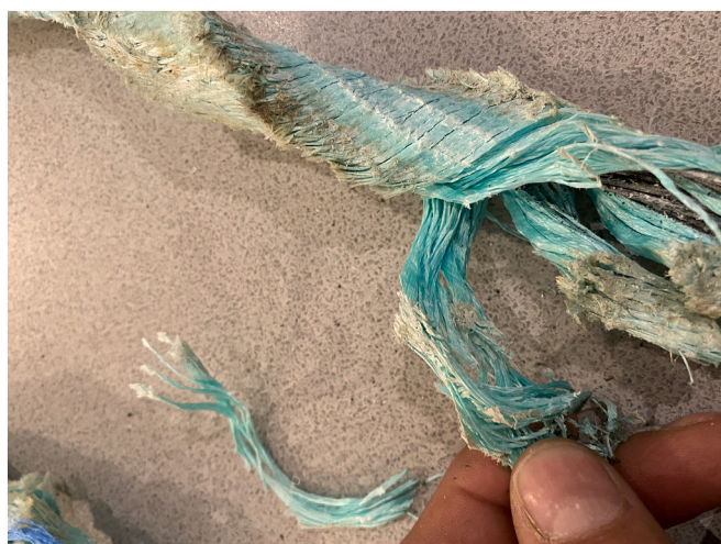
Fig. 2. Used Danish seine rope (12 months) indicating the wear after splitting the cords.
