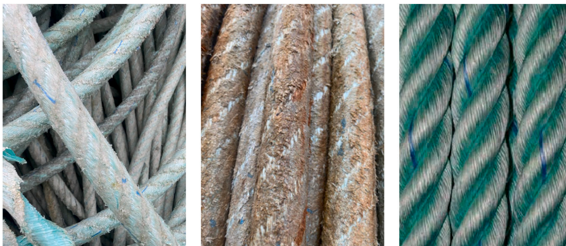
Fig. 3. Used seine ropes from vessel A (left), vessel C (middle), and new ones (right).
