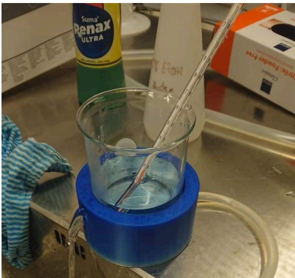
Appendix Figure 12: Set-up for the beaker for the viscosity measurements. A 3D-printed holder with tempered water flowing through it makes it possible to heat up hydrogel loaded inside the beaker. This enables measuring viscosity over time in a range of temperatures. (Martin Skipperud Skarpeid, with permission ).
