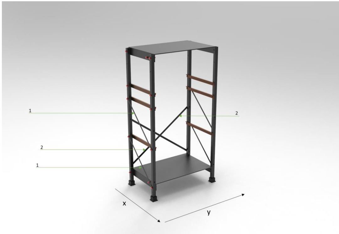
Figure 21: Bracing the structure.
