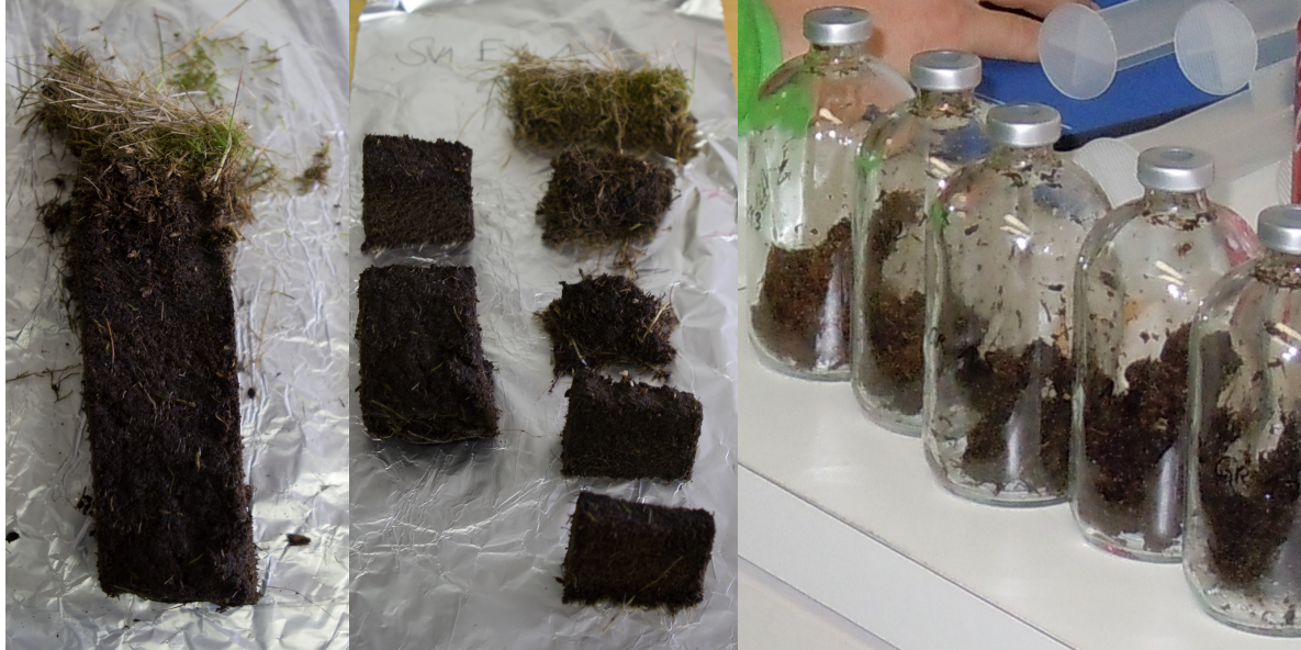
Figure 5 Microcosm preparation for Paper I. To the left is the intact peat profile. The picture in the middle shows the seven sections cut for the CH 4 oxidation potential along vertical peat soil gradients. To the right are the soils microcosms while being measured using a GC-FID.
