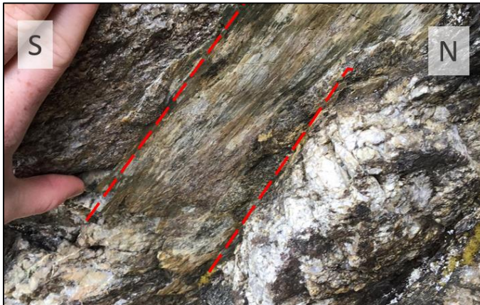
FIGURE 38: SLICKENLINES OBSERVED FROM A BRITTLE FAULT AT THE BACKSCARP REGION OF DUSNJARGA URS. DIRECTION OF MOST SMOOTH IS DOWNWARDS. PICTURE TAKEN DURING FIELDWORK IN SEPTEMBER, 2021.
