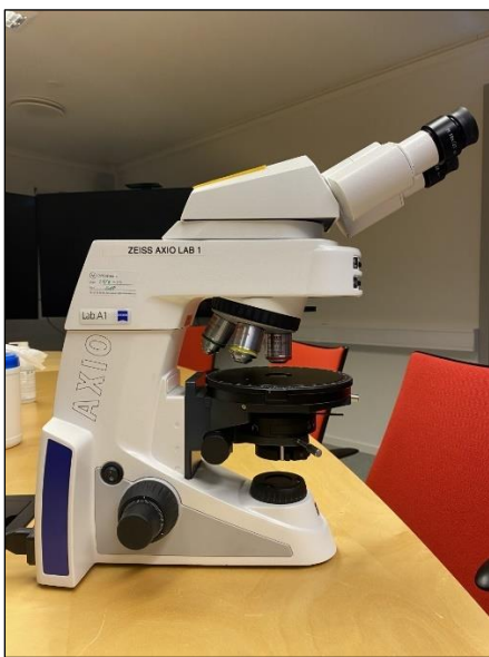
FIGURE 15: ZEISS AXIO LAB A1 MICROSCOPE USED FOR THINS SECTION STUDY.
