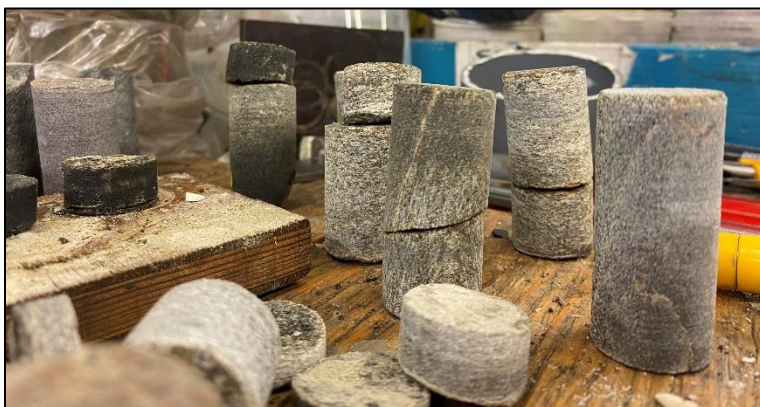
FIGURE 58: PICTURE TAKEN OF ROCK SAMPLES WHERE FAILURE OCCURRED DURING SAMPLE PREPARATION. PICTURE TAKEN AT NGI'S ROCK LAB 18/09.2021.
