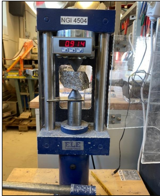
FIGURE 17: POINT LOAD TEST APPARATUS. PICTURE TAKEN AT NGI'S ROCK LAB [14.10.21].
