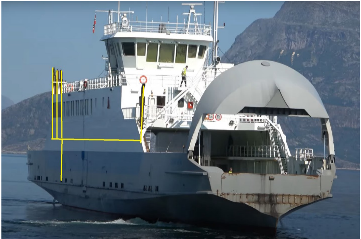
Figure 29: Connection of all the exhaust pipe of MF Lyngen at one node and routed towards capture system.
