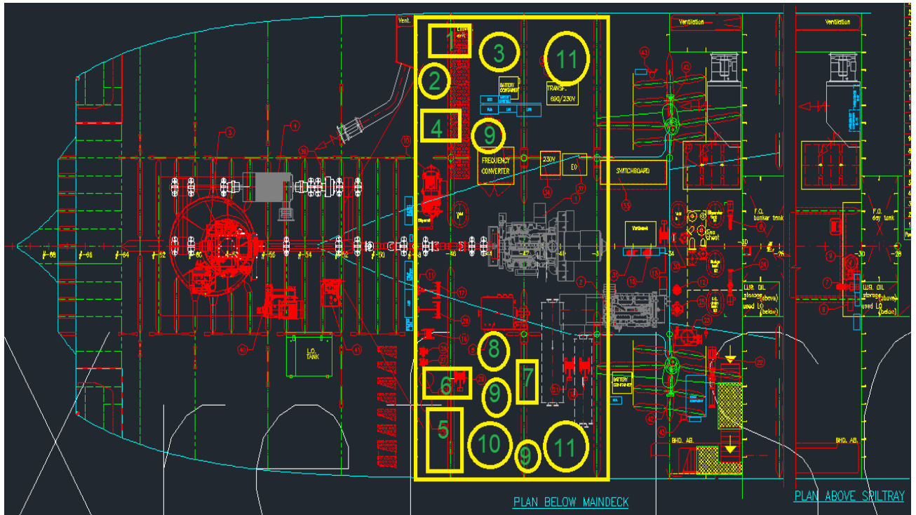
Figure 30: Top view of the MF Lyngen showing the engine room where the placement of equipment is suggested as shown (1) blower, (2) Dryer, (3) De-sublimating HX, (4) Multistage heat exchanger, (5) Refrigerant compressor, (6) flash drums, (7) Screw press, (8) Melter, (9) Pumps, (10) Distillation column, (11) CO 2 storage tanks
