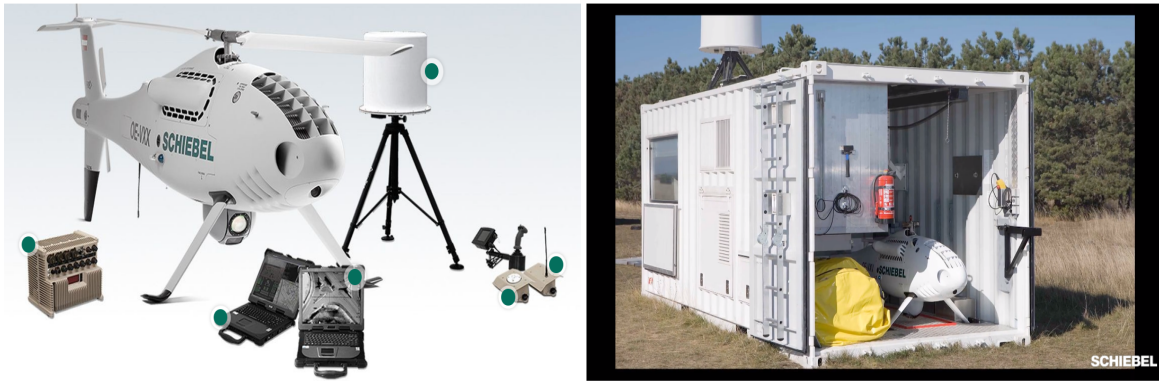
(a) The different components that comprises the GCS. (b) The GCS that can also be used as storage.
