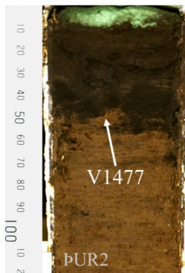
Figure 13. Visual tephra layers contained in the sediment sequences of Lake Þuridarvatn. One single tephra marker has been identified: V1477.
