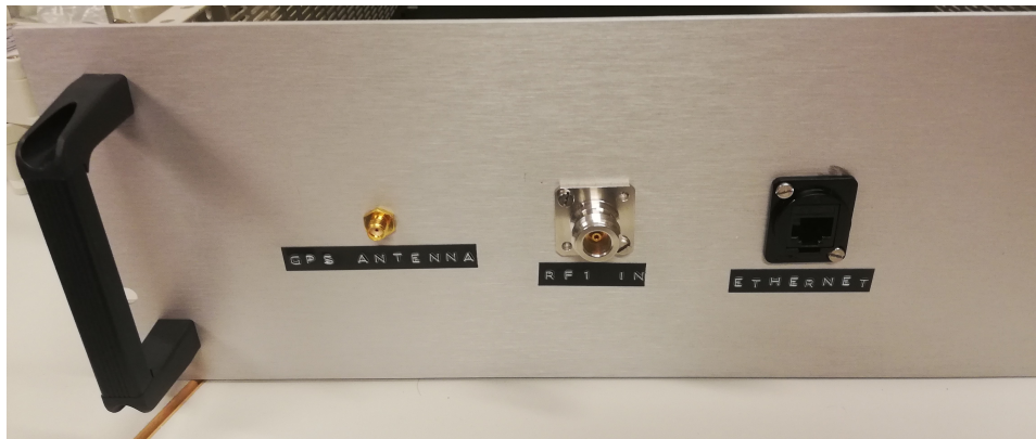
Figure 4.16: Bulkhead panel adapters installed in the front plate of the rack mounted case, labelled.
