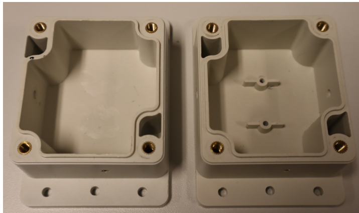
Figure 4.5: The plastic suspension brackets inside the housing were removed to clear more space for the N connector.
