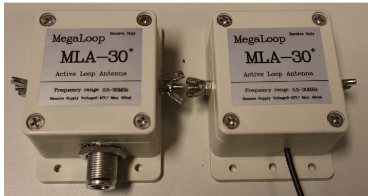
Figure 4.4: An image showing the pre-amplifier as a stock MLA-30+ (right) and the modified MLA-30+ (left).
