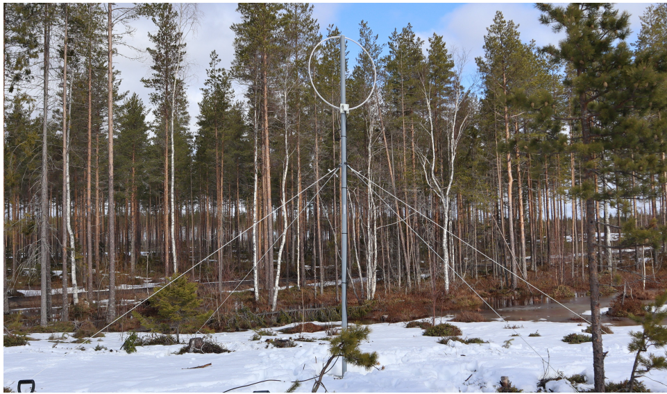
Figure 6.4: Photo of the antenna as it was installed on the Oulu site. Ground pegs were used to attach three out of four guy-wires, the last one attached to a tree.
