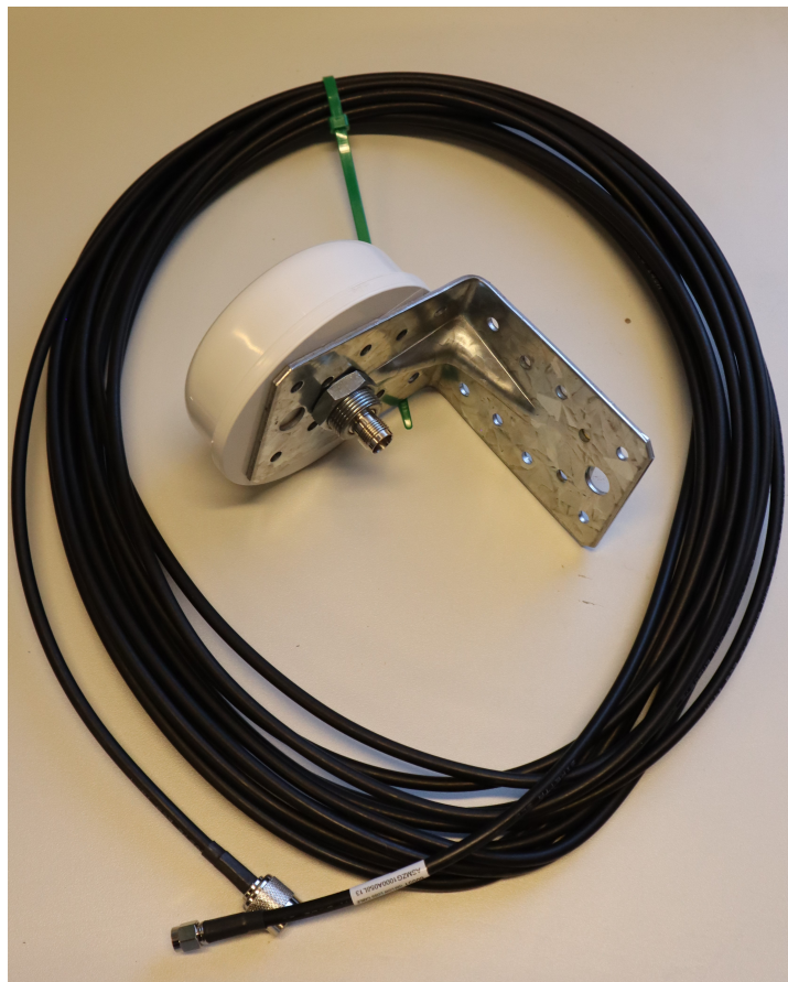
Figure 4.19: Mobilemark NT-1575-WHT antenna with 10 meter coaxial cable.
