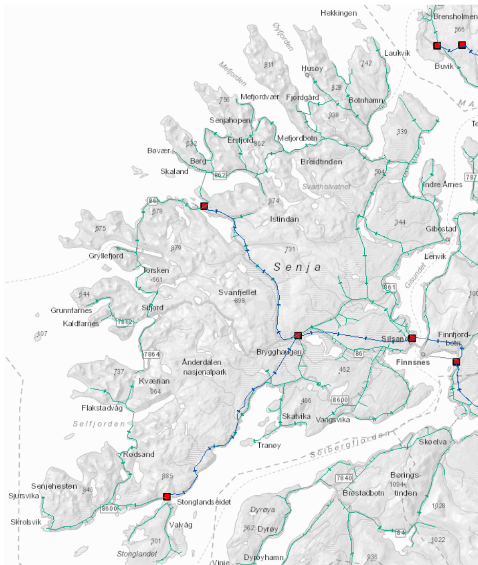
Figure 3.2: The topology of the distribution network and the hydroelectric power plants at Senja, including their reservoirs [NVE, 2021].
