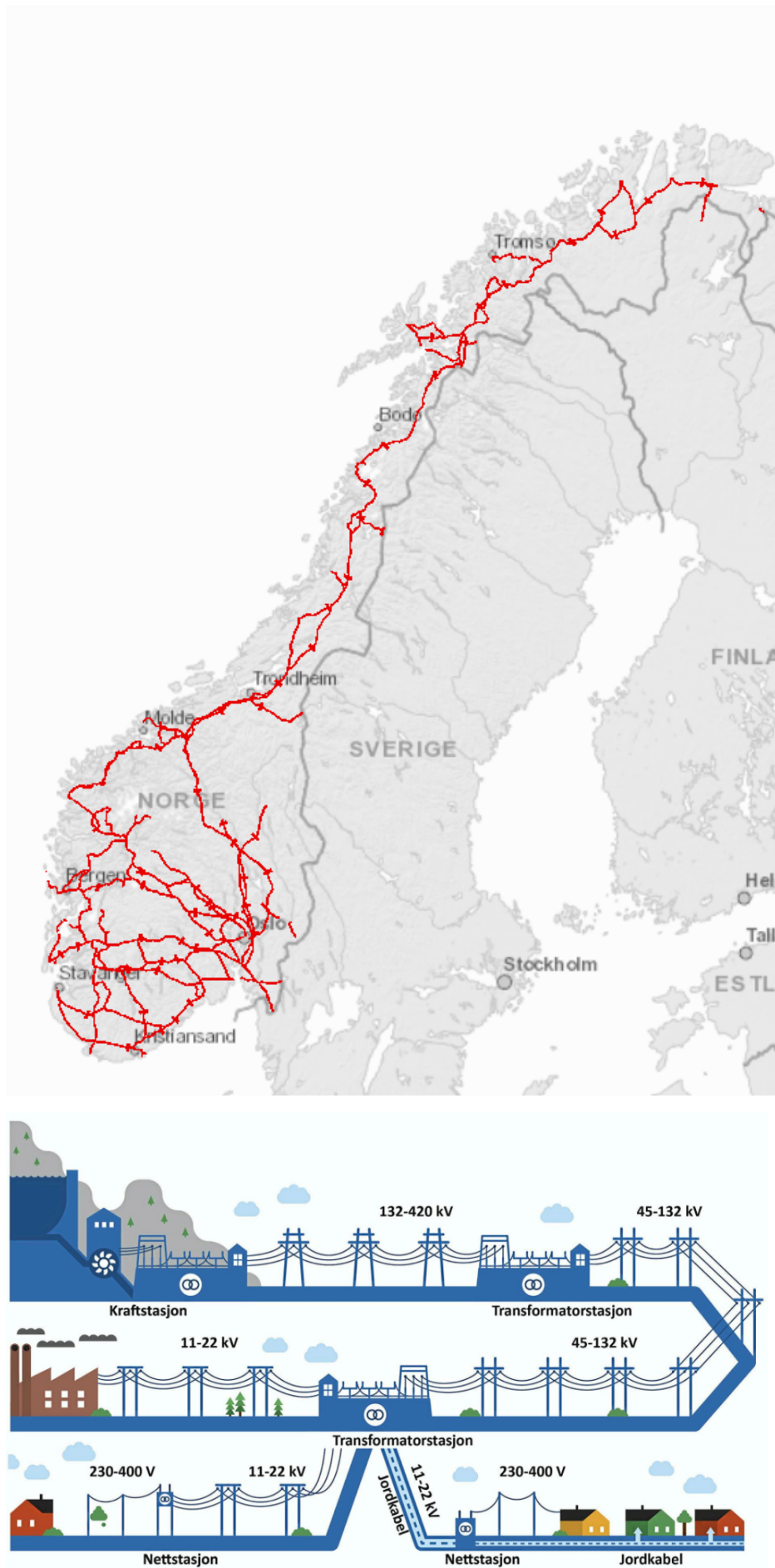
Figure 2.1: Top: The Norwegian transmission grid [NVE, 2021]. Bottom: An illustration on how the power is distributed [BKK, 2021].
