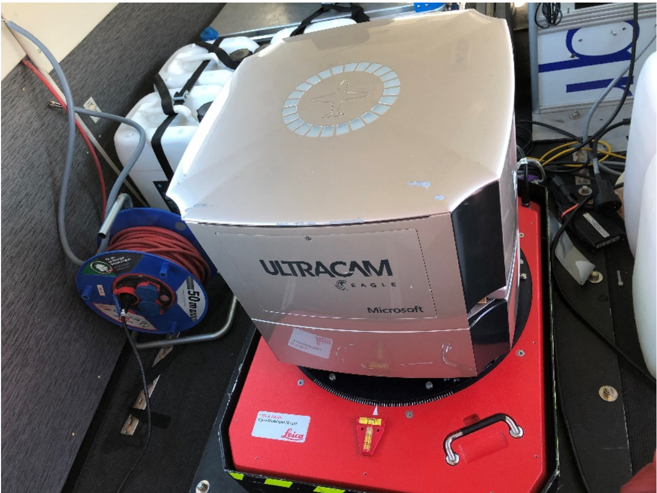
Fig. 3B. The Vexcel UltraCam Eagle Mark 3 aerial camera system mounted in the floor of the aircraft. (Photo: K. T. Nilssen).
