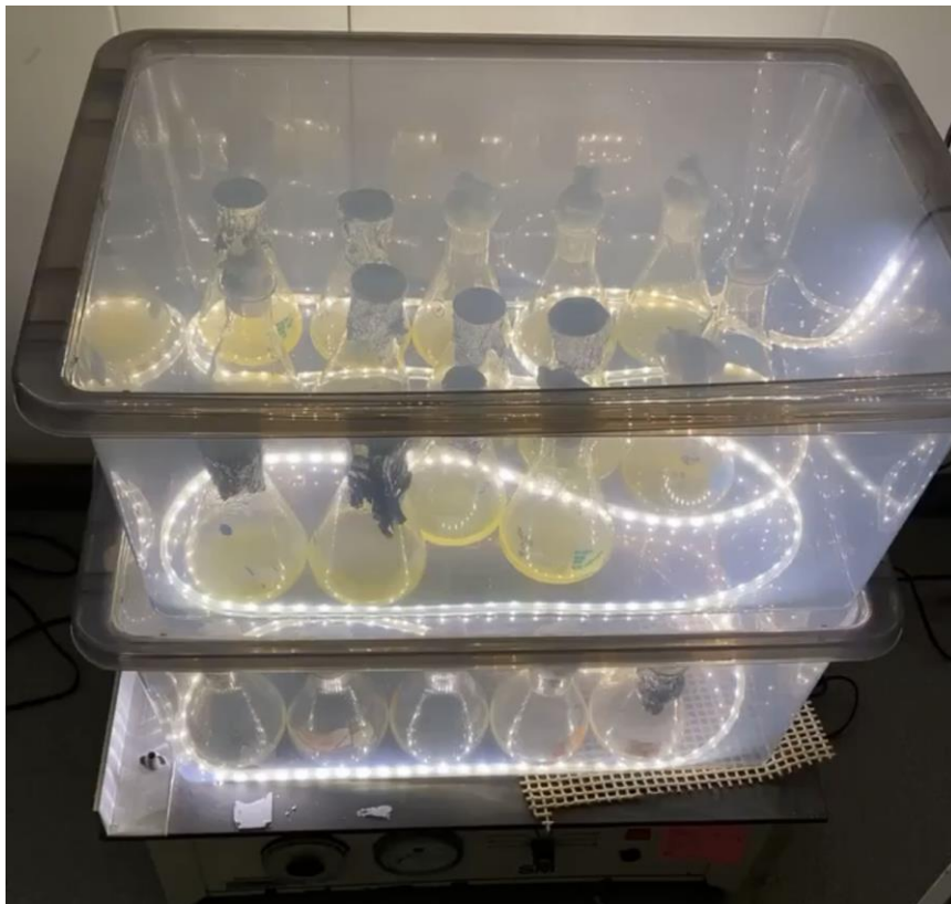
Figure 8. Microalgae growth in phototrophic conditions with f/2 media in a platform shaker.
