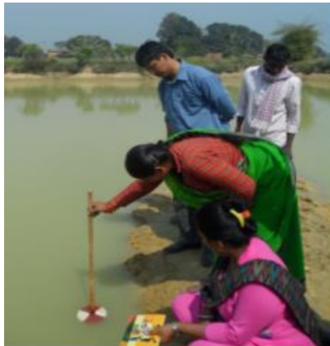
Figure 1-3 A typical modern aquaculture water monitoring operation of measuring phytoplankton density performed in ponds.
