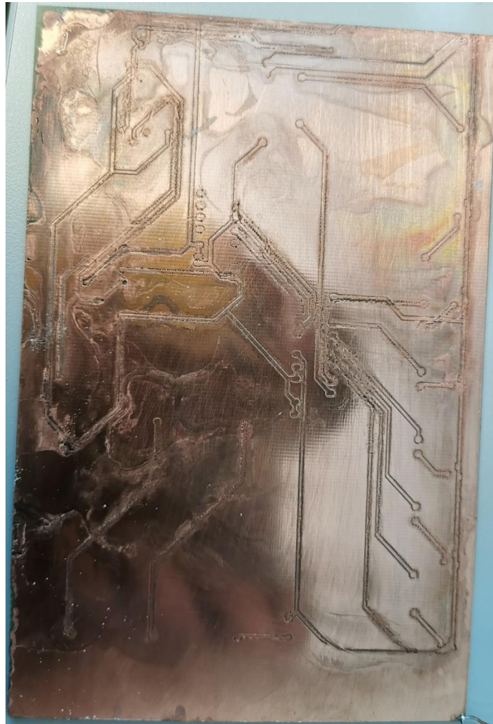
Figure 21:Initial Etch result using default Scan Velocity and low number etch passage.
