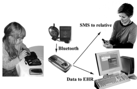
Fig. 2. Overall architecture of the no-touch wireless system for blood glucose transfer.
