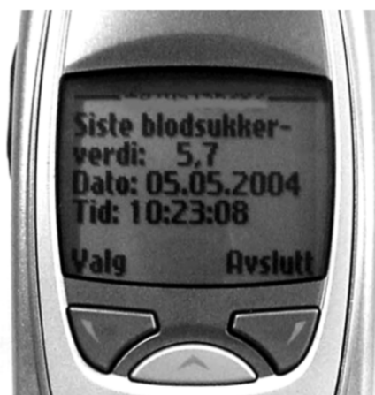
Fig. 4. Example of SMS appearing at the recipient's mobile phone. It reads: "Last blood glucose value: 5.7 (mmol/l). Date: 05.05.2004. Time: 10:23". The message may be sent to any GSM-enabled mobile phone.
