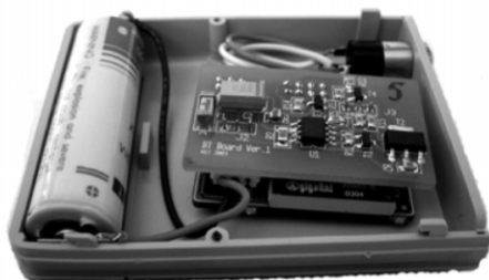
Fig. 3. Inside view of the blood glucose Bluetooth serial port adapter (battery has AA size).
