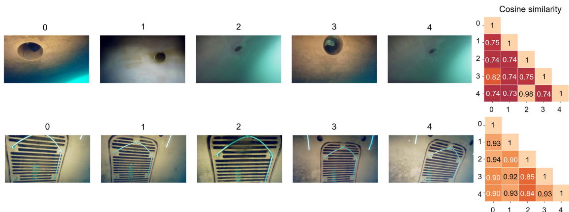
Fig. 7. Similar images of a sea chest grating and an overboard valve with corresponding pairwise Cosine similarity index.
