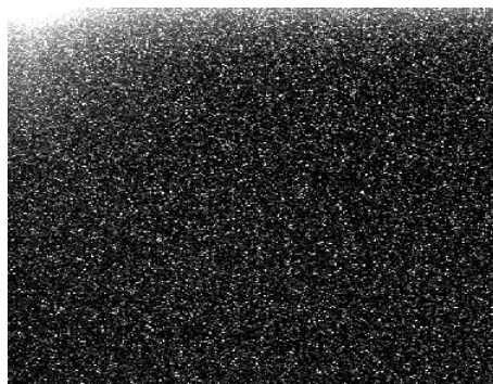
Figure 7.1: This picture is taken with an exposure time of 65 seconds and with 650 gain. It shows us the unknown noise source.
