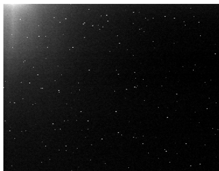
Figure 7.3: The camera had the same settings as before. The camera has been running for a while and then cooled down to 0 degrees Celsius. When the camera was cold we took this picture.
