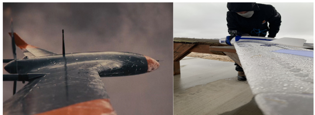
Figure 1. Ice accretion on fixed-wing UAV [13,14].
