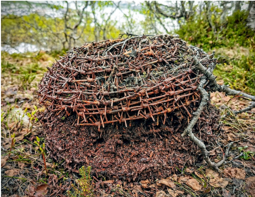
Figure 10. End of the line. A spool of barbed wire corroding into piles of iron oxide in the urban wilderness of Tromsø. The degradation of barbed wire is accelerated by humidity trapped in the vegetation. If the barbed wire hangs free in the air, it can last for decades, if not centuries.
