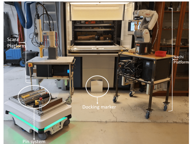
Fig. 2. The figure showcases both robot trolleys, the mobile robot with the pin system, and the marker used for docking with the mobile robot.
