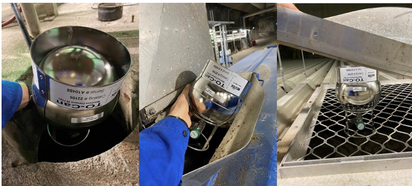
Figure 3. Sampling locations at the WWTP at Bekkelaget, from left to right sample C1, sample C2 and C3-6, samples taken in March 2022 (Photo Vogelsang, NIVA).
