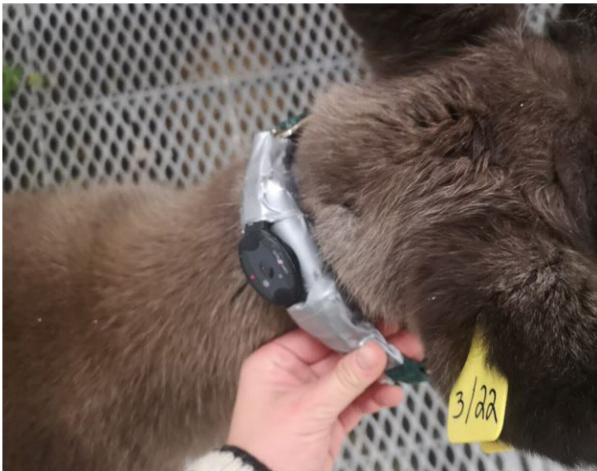
Figure 14: Actiwatch attached to reindeer harness. Attached with duct tape to ensure that it stays on the reindeer for the whole experiment.
