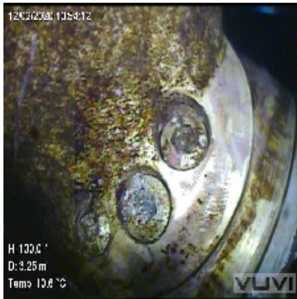
(b) The true labels for the image are "propeller" and "marine_growth." PDF and statistics can be found in figure 4.9
