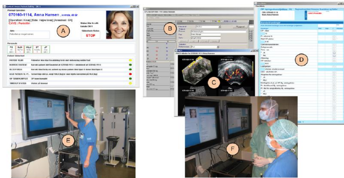
Figure 4 The CAPSIS user-interface and use: A: patient safety window, B: medical record, C: medical images, D: checklist, E: interaction, and F: reading safety status. (Bardram and Niels N 2008)
