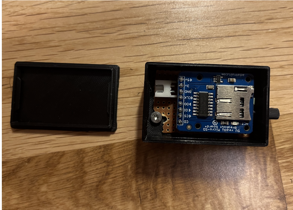
Figure 5.7: Device in the 3D printed case based on the design seen in Figure 5.6
